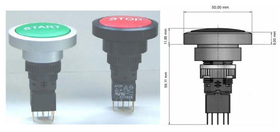
The operator is available in illuminated and non-illuminated versions, sealed up to IP65. The switch block is available in 1,2,3 or 4 poles with a latching or a momentary function.
