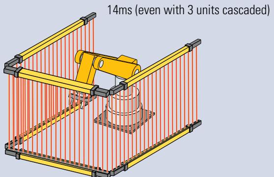
Regardless of the number of beams or the number of light curtains connected in a series, the maximum response time is 14ms! This reduces the time needed to calculate safety distances.
