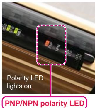
Both PNP and NPN transistor outputs are available in one light curtain.
