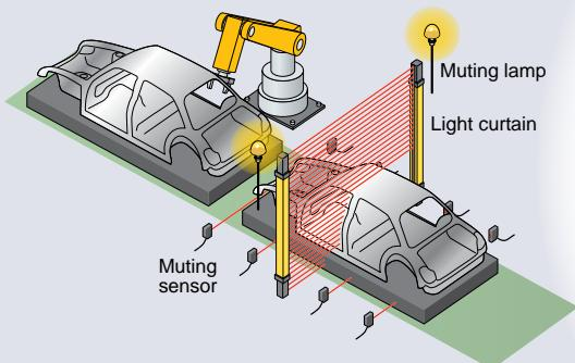
The SE4D light curtain is equipped with a muting function that causes production to stop when a person passes through the light curtain, but does not stop when an object passes through.
