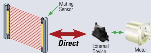
Because a special controller is not needed with the SE4D Light Curtains, a muting sensor and lamp can be directly connected reducing costs and saving installation time.
