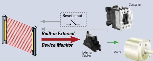
Since the SE4D light curtains have built-in EDM (external device monitoring), a safety circuit can easily be constructed without a safety relay module. As a result, the control panel can be downsized and costs reduced.
