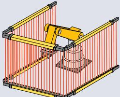
To cover "L" or "U" shaped configurations or to guard both the front and back of a machine, up to 3 light curtain sets (emitter and receiver) can be connected together in a series without any dead zones.
