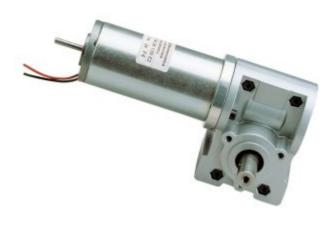
Gear motor with worm screw and standard motor  $\emptyset$  42 30 output W 24 Vdc 3700 RPM loadness, with electric noise suppressor. Driving shaft mounted on a bearing and bushing. Outlet shaft supported by two bearings with oil splash guard on the outlet side.
