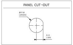
Dimensions: First dimensions are in mm while inches are shown as bracketed numbers.
