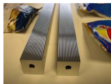
Crimped profile sealing jaws matching pair. Normal size 25mm x 300mm but can be anywhere from 5mm up to 25mm wide x 300mm long.
