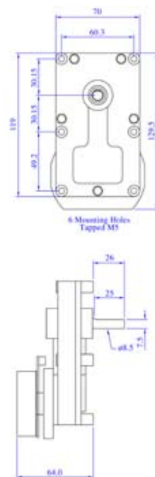
FBNB BLDC SERIES MOTOR (Figures based on 24VDC - 5V input & 0.51 amps limit)
