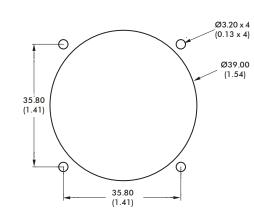
The joystick is dropped into the panel cut-out. For panel thickness of <3mm, M3 x 16 countersunk machine screws are recommended. Please note: Image (left) shows a square bezel, a circular bezel is also available for this option.
