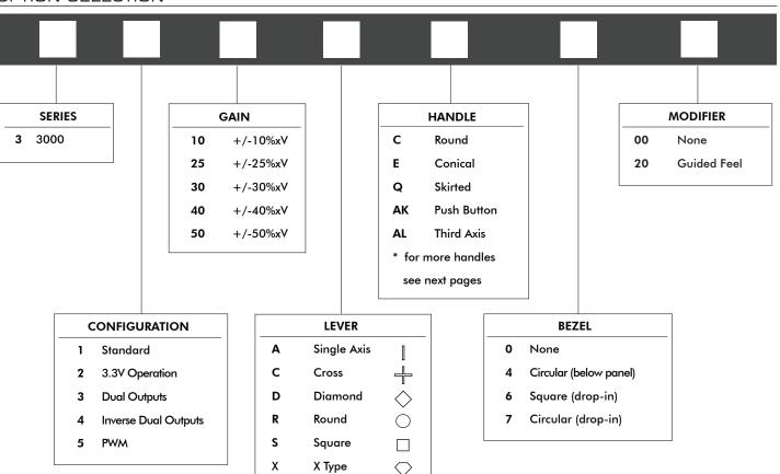
• CONFIGURATION 1 provides one proportional output per axis, a center tap reference and a separate center detect output.
