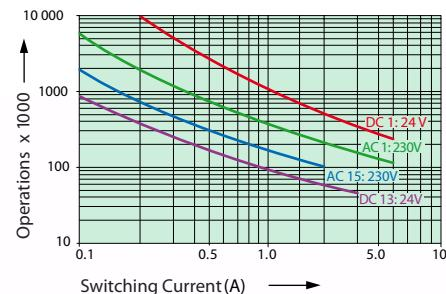
Max. Switching Characteristics (DIN EN 60947-5-1, Tab.C2):
