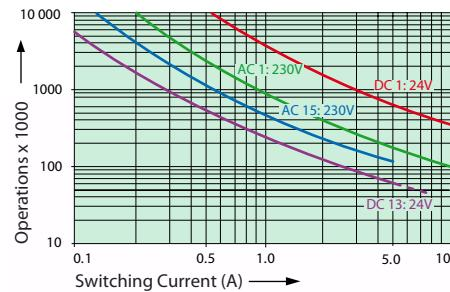
Max. Switching Characteristics (DIN EN60947-5-1, Tab.C2):
