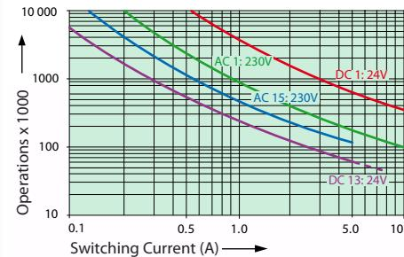
Max. Switching Characteristics (DIN EN60947-5-1, Tab.C2):
