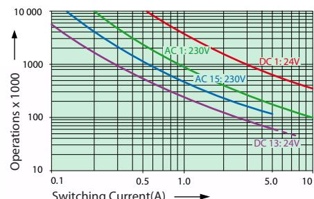
Max. Switching Characteristics (DIN EN60947-5-1, Tab.C2):
