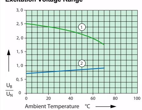
1) Max. excitation Voltage with Contact Load: ≤6A (2 Contacts)
