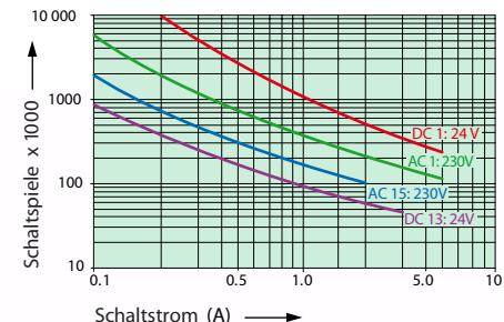
Max. Switching Characteristics (DIN EN 60947-5-1, Tab.C2):
