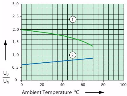
1) Max. excitation Voltage with Contact Load: <5A
