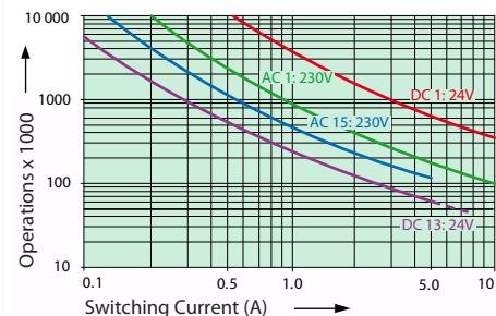
Max. Switching Characteristics (DIN EN60947-5-1, Tab.C2):
