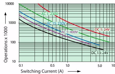
Max. Switching Characteristics (DIN EN 60947-5-1, Tab.C2):
