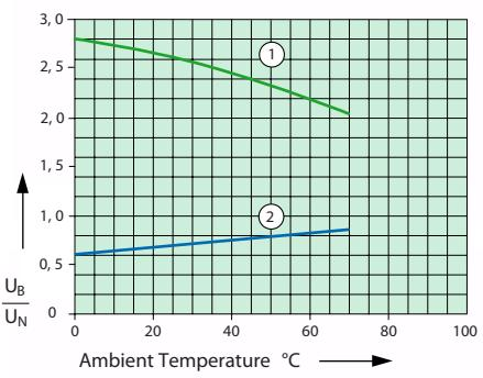
1) Max. excitation Voltage with Contact Load: <4A
