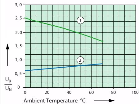
1) Max. excitation Voltage with Contact Load: <4A
