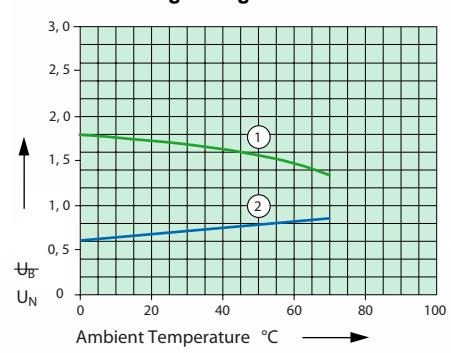
1) Max. excitation Voltage with Contact Load: ≤6A
