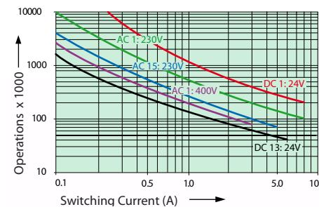
Max. Switching Characteristics (DIN EN 60947-5-1, Tab.C2):
