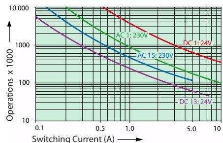
Max. switching Characteristics (DIN EN60947-5-1, Tab.C2):
