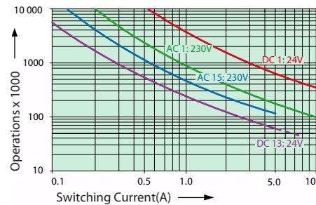
Max. Switching Characteristics (DIN EN60947-5-1, Tab.C2):
