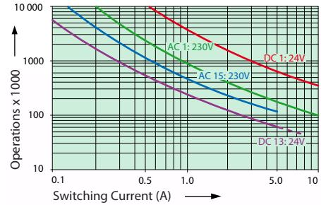
Max. Switching Characteristics (DIN EN60947-5-1, Tab.C2):
