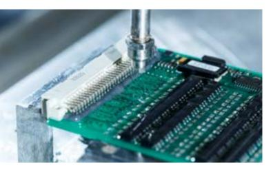
Increasing requirements for the quality, reliability and operating life of electronic assemblies as well as a growing packing density of the components make a protective coating more and more important. Constructed assemblies can be protected against moisture, dust, dirt, contamination and mechanical loads by means of special coating processes in order to prevent a functional impairment.
