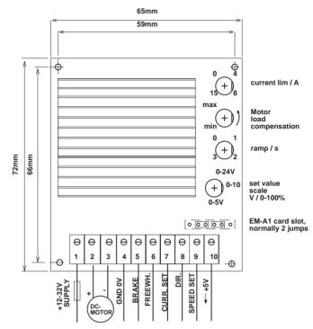
CAUTION ! Wrong polarity can damage the device. Select a fuse (1-16A) in accordance with the application.
