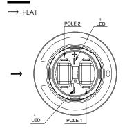
Fully illuminated pushbutton switches • bushing Ø 30 mm • momentary or latching
