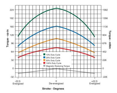
Graph 1 shows three position operation. In any mode, the armature seeks center of stroke at zero power. Applying a positive or negative voltage causes the shaft to rotate clockwise or counter clockwise. When power is removed, the restoring torque is applied to the load, or alternatively, the shaft can be driven to center under power.
