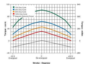
Graph 1 shows three position operation. In any mode, the armature seeks center of stroke at zero power. Applying a positive or negative voltage causes the shaft to rotate clockwise or counter clockwise. When power is removed, the restoring torque is applied to the load, or alternatively, the shaft can be driven to center under power.
