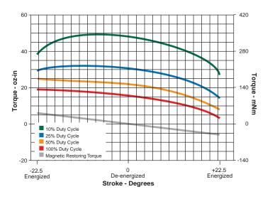
Graph 2 shows operation end-to-end. Note the high starting torque for high starting acceleration or for stopping the load by means of reverse voltage at the end of the stroke. If the device is used in a full stroke application, the load can be externally latched, detented, or biased to either end of stroke.
