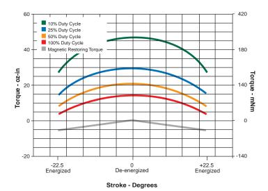
Graph 1 shows three position operation. In any mode, the armature seeks center of stroke at zero power. Applying a positive or negative voltage causes the shaft to rotate clockwise or counter clockwise. When power is removed, the restoring torque is applied to the load, or alternatively, the shaft can be driven to center under power.
