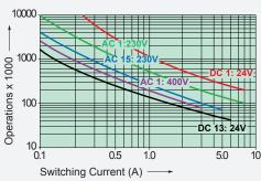
Maximal switching characteristics (DIN EN60947-5-1, Tab. C2)
