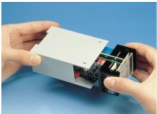
**Fast component-mounting and manufacturing** The pcb assembled with components and the terminal housing is being soldered completely in one working process.
