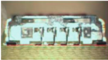
Cross Section Right Angle Male Connector
