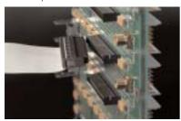
For your specific application you can decide for any board-to-board height between min. 8.0 mm and max. 14.0 mm. This is achieved by 2 styles, the standard and the low profile version.
