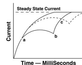
This time delay, which occurs prior to the plunger motion, is a function of the inductance and resistance of the coil, and the flux required to move the armature against the load. An increase in the magnetomotive force is created by closing the air
