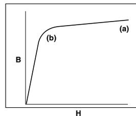
As the pole pieces are moved together or when input power is increased, the flux density of the magnetic circuit increases until the iron saturates near point (b). Beyond this point any further increase in power only serves to add heat without an appreciable increase in force or torque. By changing the iron path area, the pole shape, or the magnetic circuit material, output torque/force can be increased.
