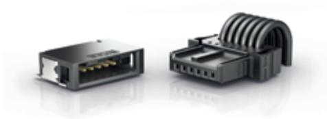
MicroBridge cable-to-board connectors were developed based on the LV214 and USCAR automotive test specifications and meet the high requirements of the automotive sector, especially in terms of connection reliability. An optional available electrical CPA (Connector Position Assurance) and Koshiri security guarantee secure and proper connection.
