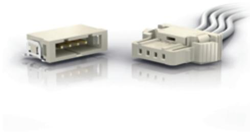
The single- and double-row iBridge Ultra connectors with SMT and dip solder terminals represent an expansion of the proven iBridge connector solution with a 2 mm pitch that is compatible for crimp terminations and wire cross sections of AWG 22/24. The high retention force guarantees reliable mating, even in demanding environments subjected to strong vibrations.
